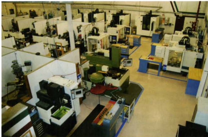
In the tool room at PTI Engineered Plastics, functional prototypes are created to support customers' early production needs, also known as bridge tooling. Functional prototypes meet aggressive market entry targets with tools that provide high repeatability and molded-in quality without compromising long-range goals.
